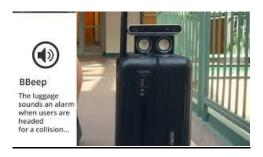
Smart Suitcase BBeep has been developed which warns impending collisions with help of a navigation mobile application NavCog. The blind users can be well assisted while navigating in airports independently and safely.
